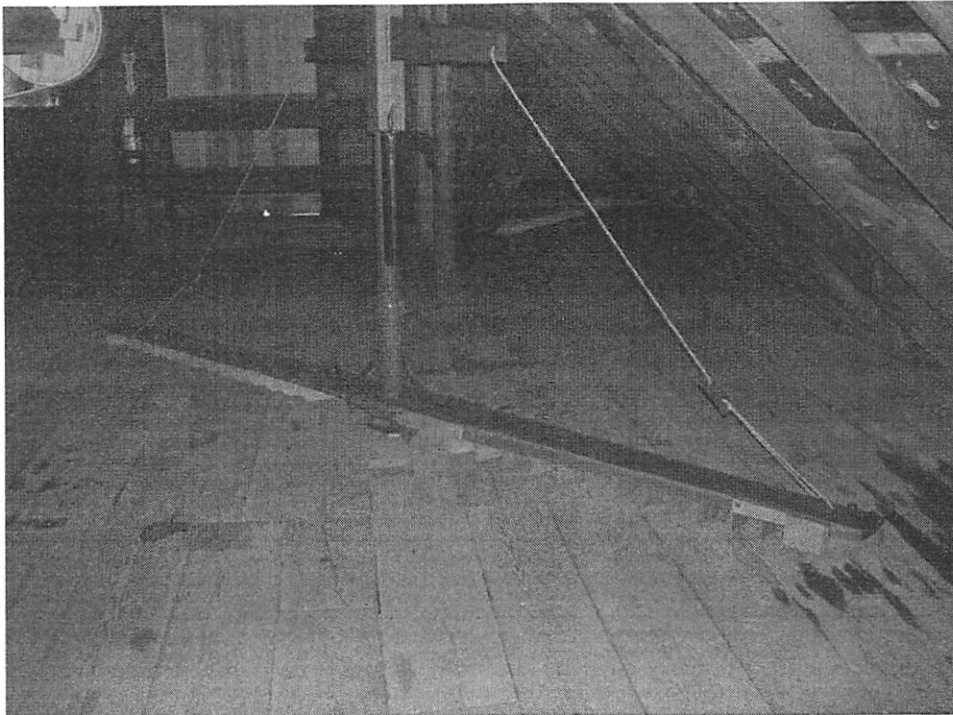
Figure 2: An example of Oliver Evans' hopper boy, found in Yates Mill. Prior to Evans' invention, millers would have hired a young boy to spread the wheat meal out manually.
